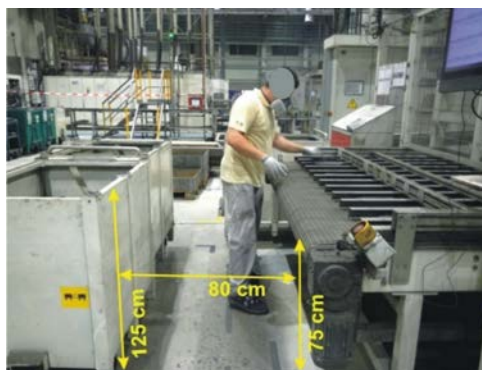
FIG. 1. Conveyor belt, trolley, workspace dimensions
