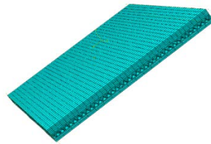
FIG. 9. Finite element model for multilayer plate
