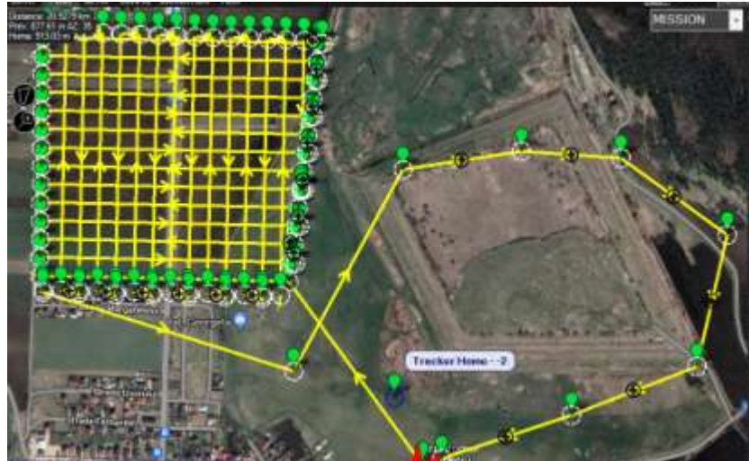
FIG. 7 Defined flight path with landing, survey grid and landing attached.
