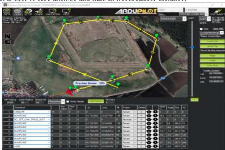
FIG. 5 Landing path generated in Mission planner
