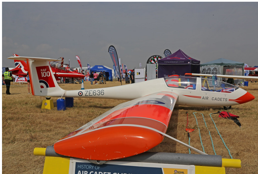
FIG. 2. Royal Air Force's Grob T1 Viking (Military version of Grob 103) Two-Seater Training Glider in RAF RIAT Air show ( https://hiveminer.com/Tags/glider%2Cmilitary , Micheal Hibbins)
