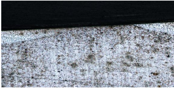
FIG.1. OLC 45 steel improved and superficial hardened (laser CO2) superficial layer +ZIT; Nital Attack 200:1
