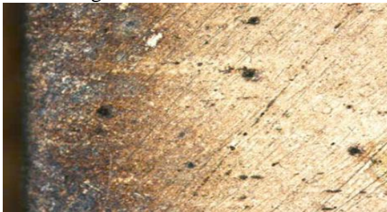
FIG.3. OLC45 improved steel and superficial hardened with electron beam. Nital Attack 200:1
