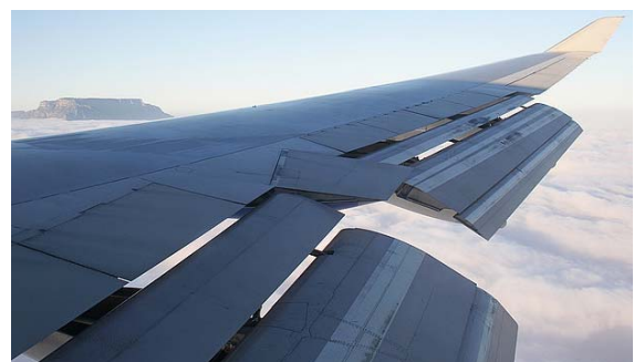
Fig. 1.6 Multiple slotted flaps - Boeing 747, [5]
