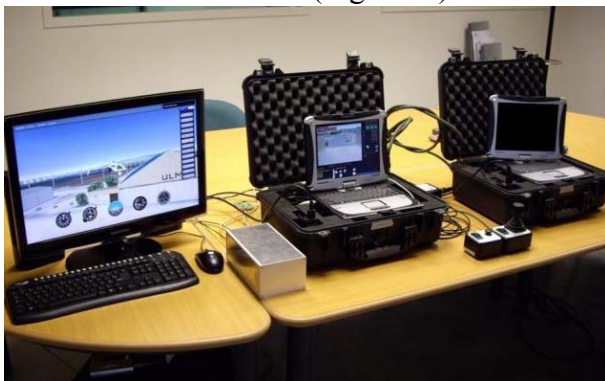
Figure 2.: Training device providing simulation for Nano, Micro and Mini category UAVs.
