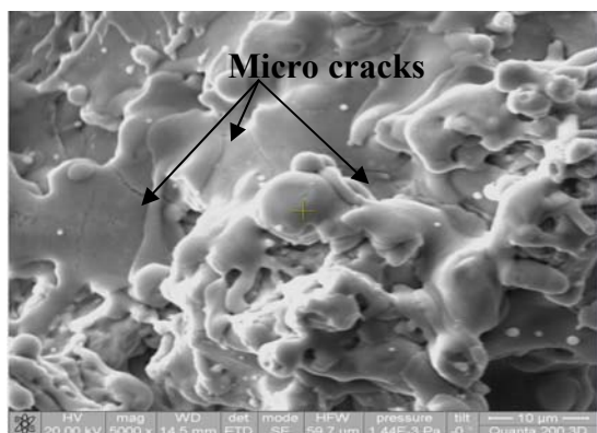
Fig.5. SEM image of the coatings surface at a magnification of 5000X
