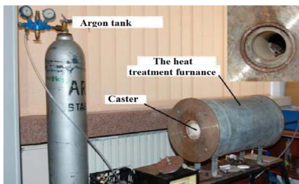
Fig. 1. The electric furnace installation
