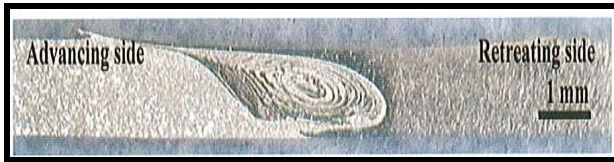
Obr. 3 Transversal cross section of a weld [1]
