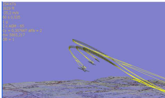
Fig. 8 Calculation of aircraft manoeuvrability using mathematical simulation
