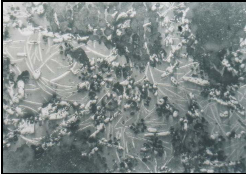
Fig. 1.10. Sample appeal \text{FeCl}_3 + \text{HCl} chemical mass-R1 ceramic impregnated with Cu, marginal zone; 250X
