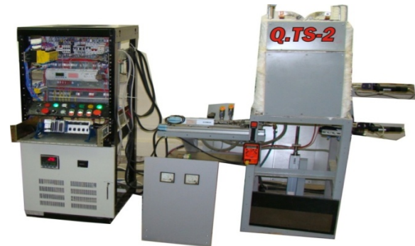
Fig.1. QTS2-Installation for material testing in extreme thermal conditions
