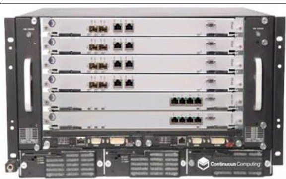
Fig. 4 The experimental configuration – front view of the installed ATCA 40G platform
