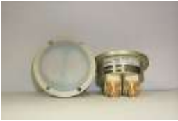
Four E/J band antennas are installed at quadrant locations around aircraft.
