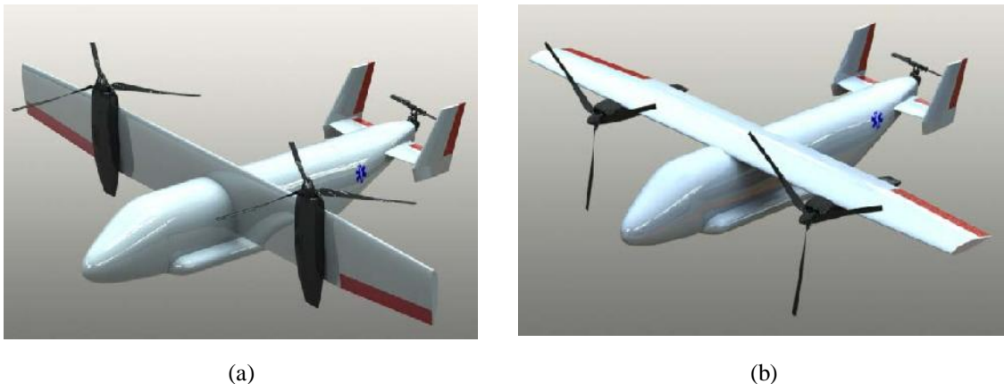
FIG. 8. Flight configuration of the ambulance-delivery UAV (a) helicopter configuration mode (take off/ landing/ hover) (b) airplane configuration mode
