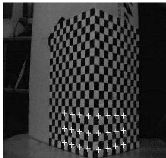
FIG.2. The calibration object and resulting calibration points.
