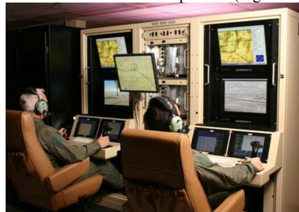
Figure 4.: Simulator which provides training to a medium category UAV.
