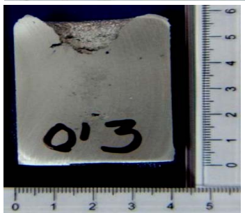
Fig. 3 Blister aspect for different situations a- non-vibrated; b- the vibration of melted alloy (only in pot, before casting)
