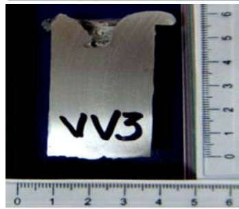
Fig. 4 Examples of section blisters a- solidified under the influence of vibration after casting until solidification; b- vibrating the alloy in the pot and during casting until solidification.
