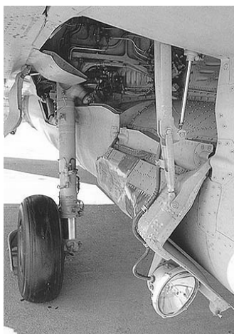
Figure 4: MiG29 main landing gear
