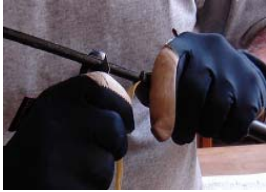
Fig. 2 - the optical fiber cable after elimination of the protective outer casing
