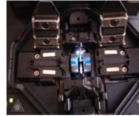
Figure 5 - guiding mechanism, welding equipment and electrodes microcamerele fiber
